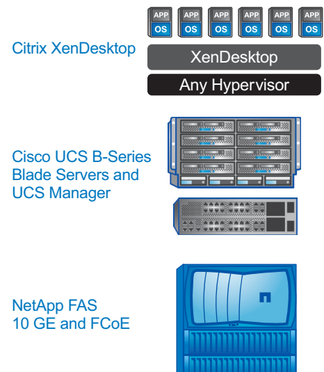
Figure 1. FlexPod DataCenter with Citrix XenDesktop, a prevalidated reference architecture combining NetApp storage, Cisco Unified Computing System (UCS) servers, and Cisco Nexus switches.
