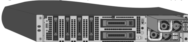
Figure 4. Inserting the Replacement DC Power Supply
