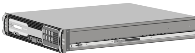
Figure 1. Attaching inner rails
