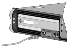
Figure 1. Inserting an Ethernet cable
