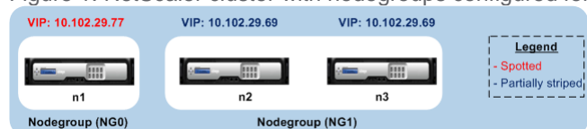
Figure 1. NetScaler cluster with nodegroups configured for spotted and partial-striped configurations
