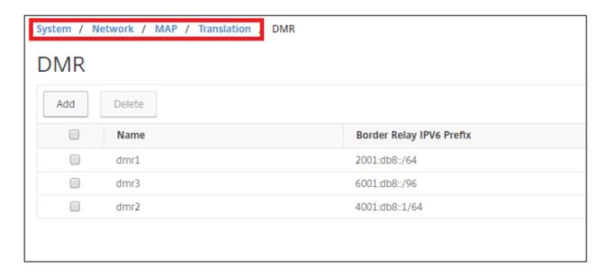
Default Mapping Rule prefix(DMR) is used to generate source IPv6 address towards CE as part of NAT46 translation on BR. For generating source IPv6 address towards CE, Border Relay IPv6 prefix is used. Details of DMR name and Border Relay IPv6 prefix has to be filled as shown below.
