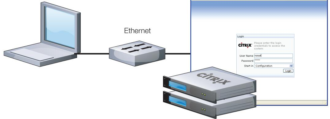
In a High Availability deployment, one Application Switch actively accepts connections and manages servers, while the second monitors the first. If the first Application Switch quits accepting connections for any reason, the second Application Switch takes over and begins actively accepting connections. This prevents downtime and ensures that the services provided by the Application Switch will remain available even if one Application Switch ceases to function.
